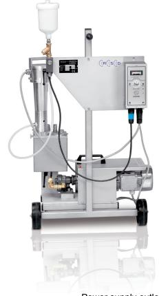
Type of machine CP-80-63-02 Control accurancy +/- 0,1 seconds
